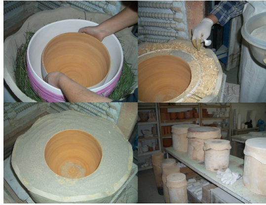
Figure 2. Placing the forms inside of the Saggar Boxes with Pine Needles, Saw Dust and Sand (Mehmet Tüzüm KIZILCAN)
