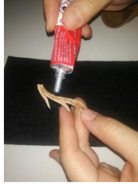
Figure 14. Sticking the cut leather (pattern model) on the fabric to be processed with adhesive (authors' photograph, 2019).
