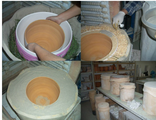
Figure 2. Placing the forms inside of the Saggarr Boxes with Pine Needles, Saw Dust and Sand (Mehmet Tüzüm KIZILCAN)
